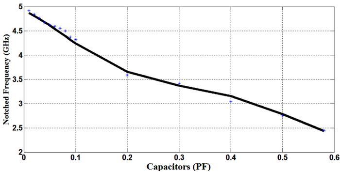
**Figure 6.** Fitting curve for the effect of lumped capacitor values on filter notch frequency response.
