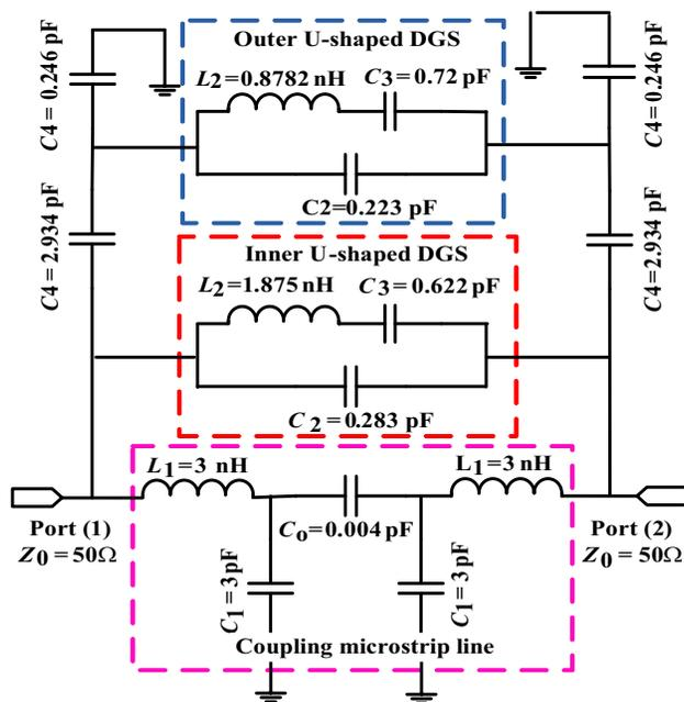
**Figure 2.** Equivalent circuit of the proposed UWB bandpass filter with notch band implementation by using 2U-DGS by ADS simulator [21].
