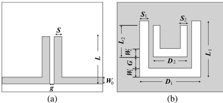
**Figure 1.** (a) Top view of the structure. (b) 2U-shaped DGS structure on the ground plane.
