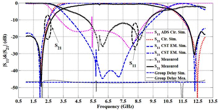
**Figure 15.** EM-simulated, equivalent-circuit modelled and measured  $S$ -parameters of UWB BPF with PIN diode in outer U-DGS.
