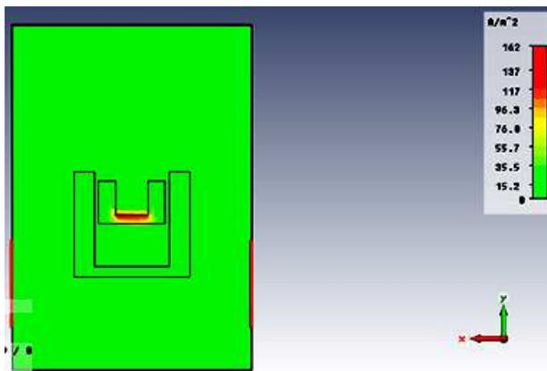
**Figure 3.** Simulated current distribution at 5.5 GHz for the bottom view.
