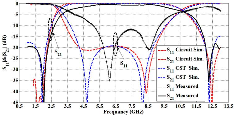
**Figure 10.** EM-simulated, equivalent-circuit model and measured  $S$ -parameters of UWB BPF with capacitor 22 pF in outer U-shaped DGS.
