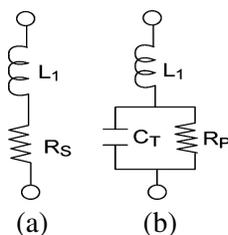
**Figure 12.** Equivalent circuit for PIN diode. (a) Forward bias. (b) Reverse bias.
