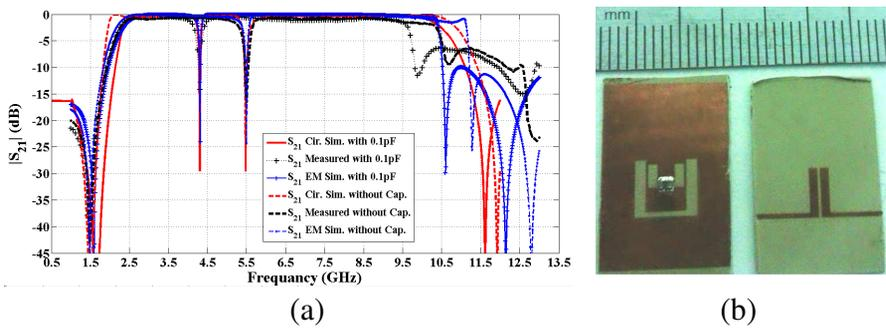
**Figure 8.** Simulated, equivalent-circuit model and measured  $S_{21}$  of notched band in UWB BPF with/without capacitors of 0.1 pF in inner U-DGS. (b) Photograph of fabricated filter.
