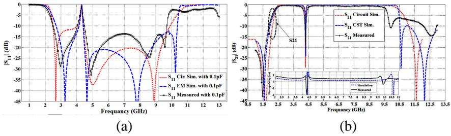
**Figure 7.** Simulated, equivalent-circuit modelled and measured  $S$ -parameters of notched band in UWB BPF with capacitor 0.1 pF in inner U shaped DGS. (a)  $S_{11}$ , and (b)  $S_{21}$ .
