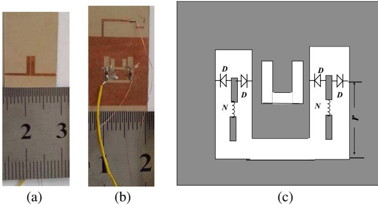
**Figure 16.** (a) Photograph of the final circuit top view, (b) bottom view, and (c) the filter with pads for switches soldering.
