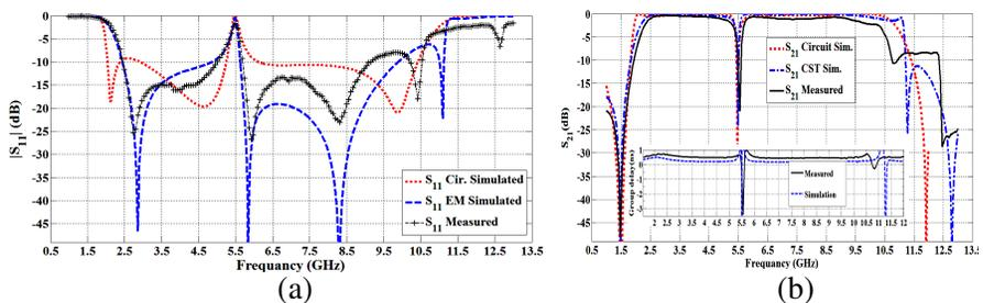
**Figure 4.** CST EM-simulated, equivalent-circuit modeled and measured  $S$ -parameters of the proposed 2U-UWB BPF. (a)  $S_{11}$ , and (b)  $S_{21}$ .
