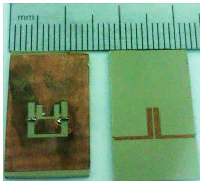
**Figure 11.** A photo for the fabricated 2U-shaped DGS filter with two lumped capacitors 22 pF each loaded in outer U-DGS.
