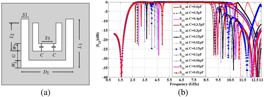
**Figure 5.** (a) Bottom view showing the 2U-shaped DGS with lumped capacitors. (b) Effect of lumped capacitor values on filter notch frequency response.
