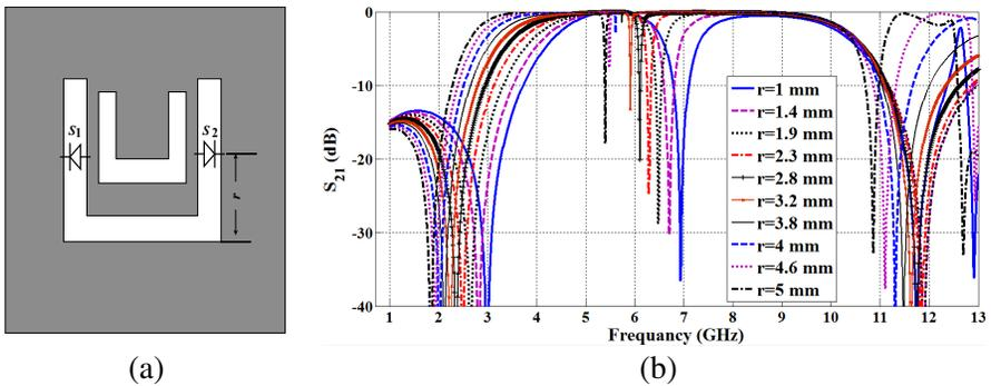
**Figure 13.** (a) Bottom view of 2U-DGS BPF with PIN diodes. (b) Effect of distance ( $r$ ) of PIN diode position on filter notch frequency response.
