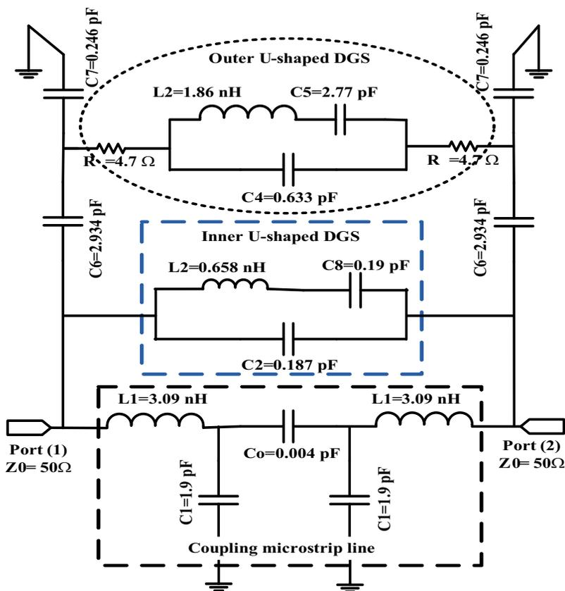
**Figure 14.** Equivalent circuit of the proposed UWB BPF with reconfigurable notch band implementation by using RF PIN diode in outer U-DGS by ADS simulator [21].
