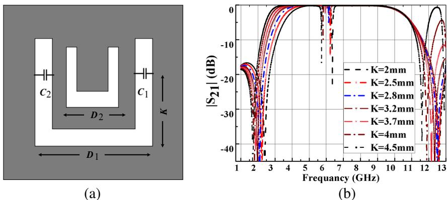
**Figure 9.** (a) Bottom view of 2U-DGS BPF. (b) Effect of distance ( $K$ ) of lumped capacitor value of 22 pF on filter notch frequency response.
