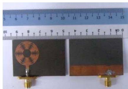
Figure 10. Photograph of the realized Fractal antenna.
