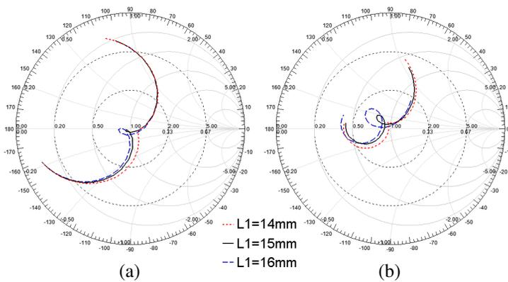
**Figure 6.** Measured input impedance for the proposed antenna at (a) 1.55–1.7 GHz and (b) 2.42–2.58 GHz.
