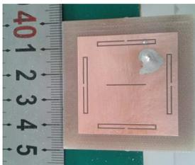
**Figure 7.** Photo of the fabricated antenna.
