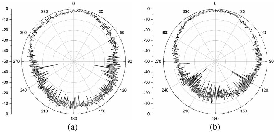
**Figure 11.** Measured radiation patterns against frequencies for the proposed antenna at (a) 1.616 GHz and (b) 2.492 GHz.
