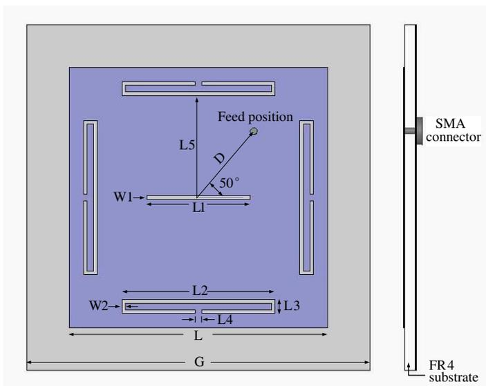
**Figure 1.** Geometry of the dual-band circularly-polarized antenna.
