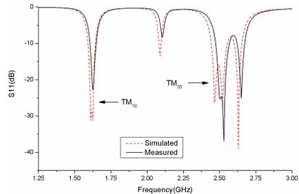
**Figure 8.** Simulated and measured results of  $S_{11}$  for the proposed antenna.
