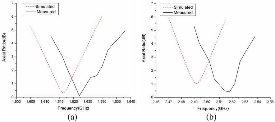
**Figure 9.** Axial-ratio against frequencies for the proposed antenna.
