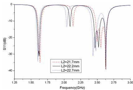
**Figure 4.** Simulated results of  $S_{11}$  for the proposed antenna with different  $L2$ .
