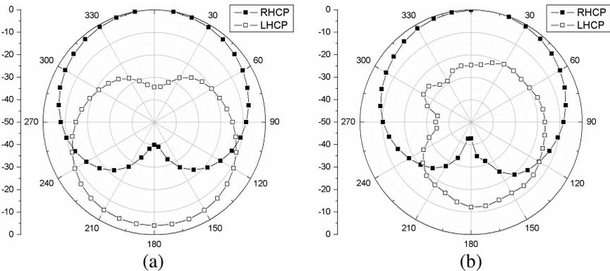
**Figure 10.** Simulated radiation patterns against frequencies for the proposed antenna at (a) 1.616 GHz and (b) 2.492 GHz.
