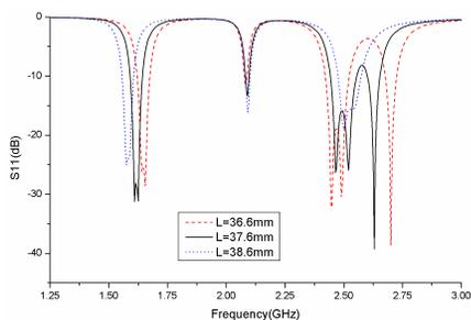
**Figure 3.** Simulated results of  $S_{11}$  for the proposed antenna with different  $L$ .
