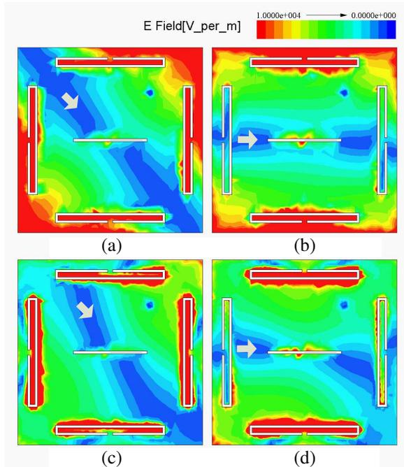
**Figure 2.** Distributions of simulated electric field. (a) 1.616 GHz@ $t = 0$ , (b) 1.616 GHz@ $t = T/8$ , (c) 2.492 GHz@ $t = 0$ , (d) 2.492 GHz@ $t = T/8$ .
