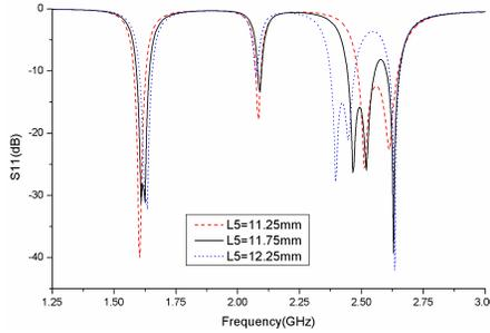
**Figure 5.** Simulated results of  $S_{11}$  for the proposed antenna with different  $L5$ .
