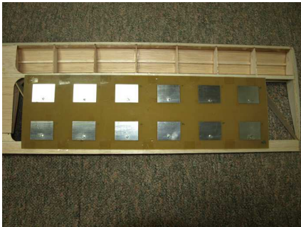
Figure 9. The 2 \times 6 array attached to the wing structure of the UAV.
