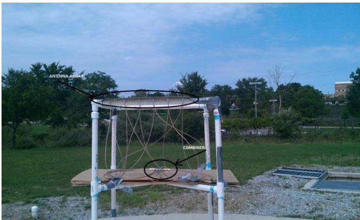
Figure 15. Antenna range setup (Oakland University, Michigan, USA).
