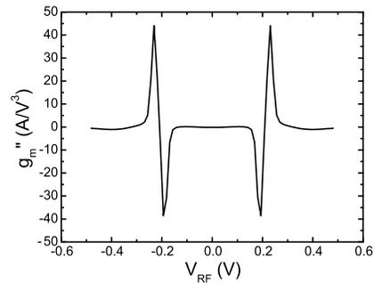
**Figure 7.**  $g_m''$  phenomenon of the current-reuse bulk-controlled mixer.
