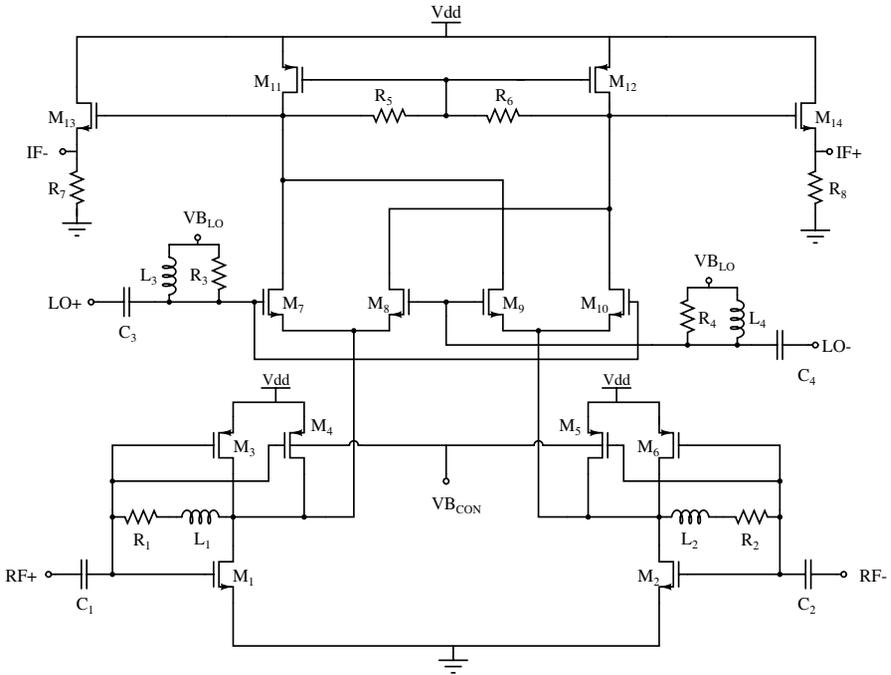
**Figure 5.** Schematic of the current-reuse bulk-controlled mixer.
