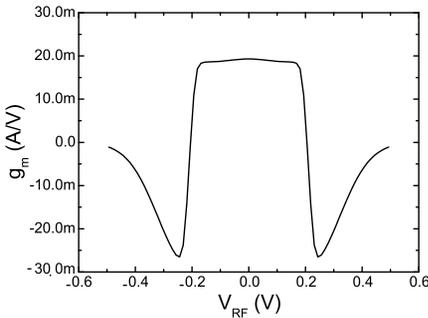
**Figure 6.**  $g_m$  characteristic of the current-reuse bulk-controlled mixer.
