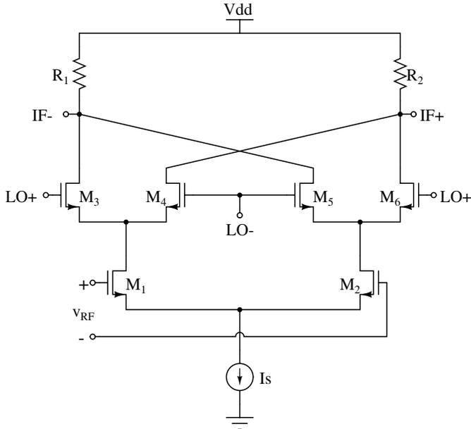
Figure 1. Schematic of the Gilbert cell mixer.
