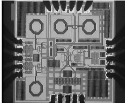
**Figure 16.** Photograph of the current-reuse bulk-controlled mixer.
