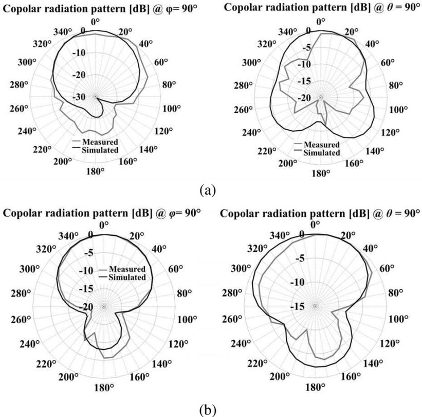
**Figure 5.** Experimental data obtained for the copolar radiation pattern of the antennas illustrated (a) in Fig. 3(a) and (b) in Fig. 3(b).
