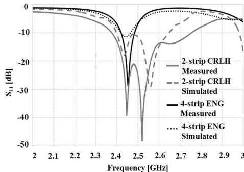
**Figure 4.** Reflection coefficient of the 4-strip ENG (i.e., the antenna illustrated in Fig. 3(a)) and of the 2-strip CRLH (i.e., the antenna illustrated in Fig. 3(b)).
