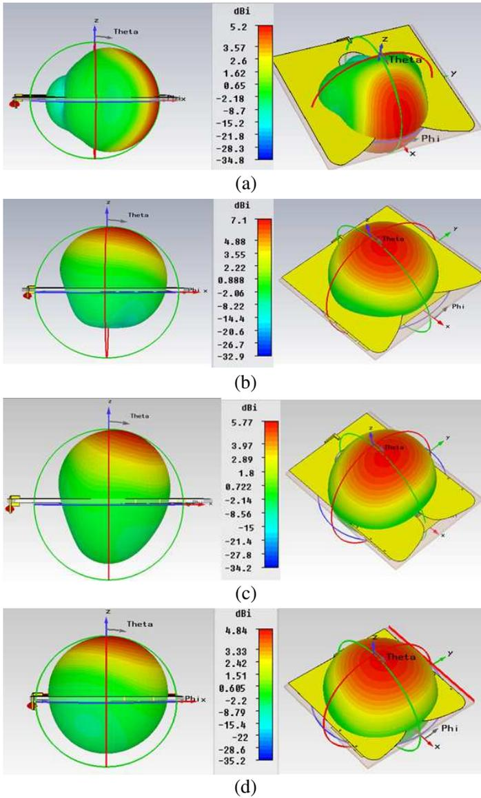
**Figure 2.** 3D simulated radiation pattern of the proposed antenna: (a) conventional Vivaldi, (b) 4-strip ENG illustrated in Fig. 1(b), (c) 4-strip CRLH, (d) 2-strip CRLH illustrated in Fig. 1(d).
