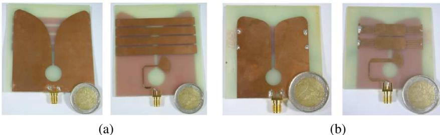
**Figure 3.** Photographs of the fabricated antennas: (a) 4-strip ENG (see Fig. 1(b)), (b) 2-strip CRLH (see Fig. 1(d)).
