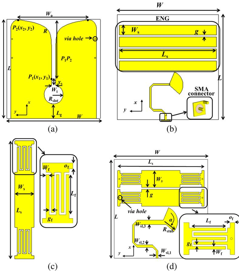
**Figure 1.** Geometry of the proposed antenna. (a) Front-view, (b) 4-strip ENG back-view, (c) 4-strip CRLH: single strip, (d) 2-strip CRLH back-view.
