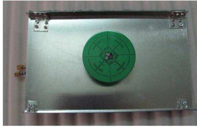
**Figure 2.** Photograph of proposed antenna.
