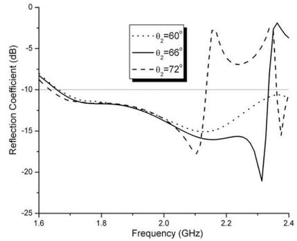
**Figure 7.** Simulated reflection coefficient, varying  $\theta_2$ .
