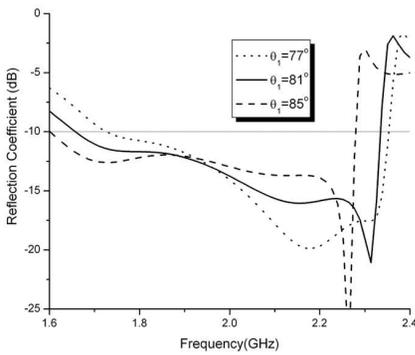
**Figure 6.** Simulated reflection coefficient, varying  $\theta_1$ .
