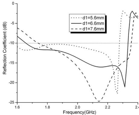
**Figure 8.** Simulated reflection coefficient, varying  $d1$ .
