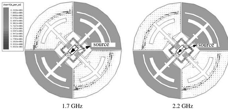
**Figure 5.** The simulated current distribution on the surface of the antenna.
