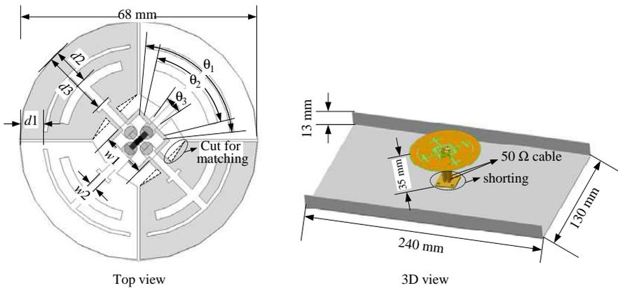
**Figure 1.** Geometry of proposed antenna.
