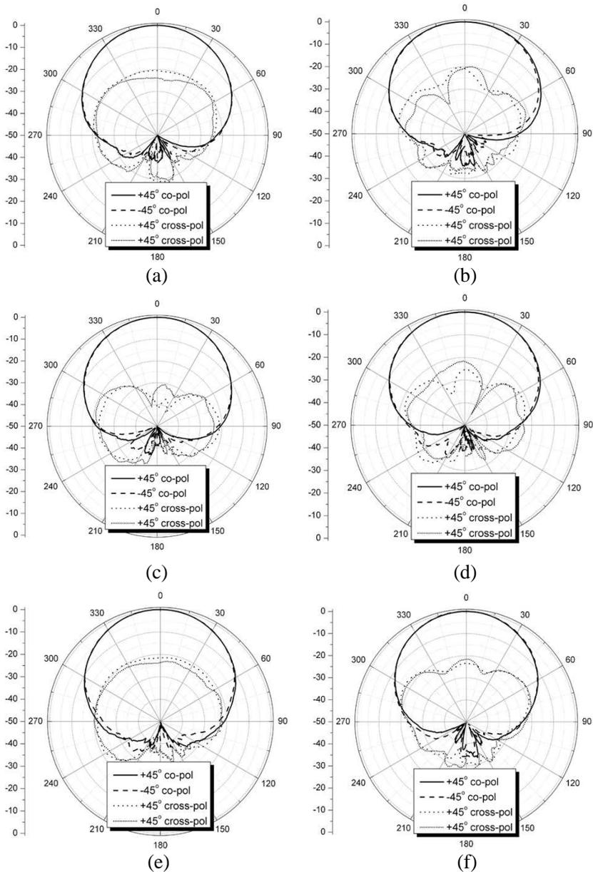
**Figure 4.** Measured radiation patterns of proposed antenna. (a) 1.7 GHz, azimuth plane. (b) 1.7 GHz, elevation plane. (c) 1.95 GHz, azimuth plane. (d) 1.95 GHz, elevation plane. (e) 2.2 GHz, azimuth plane. (f) 2.2 GHz, elevation plane.
