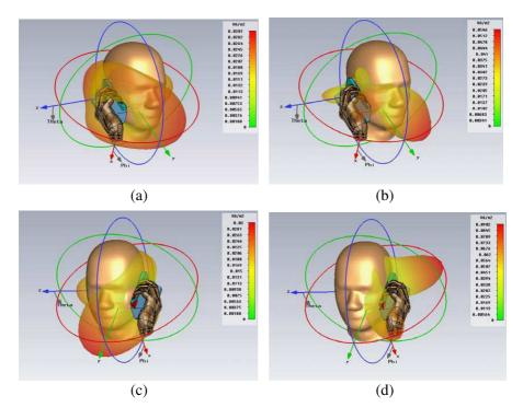
Figure 5. (a) Radiation patterns in the talking position for position 3 at (a) 0.8 GHz, (b) 1.8 GHz with the right hand and at (c) 0.8 GHz, (d) 1.8 GHz with the left hand.
