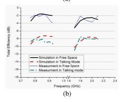
Figure 12. (a) The measurement setup and (b) the measured and simulated total efficiency of our proposed antenna.
