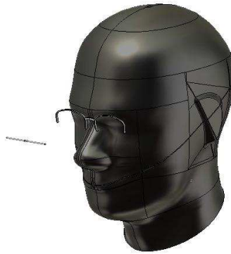
Figure 8. Diagram of SAM phantom head-worn, metal-frame spectacles replaced the metal rod exposed to RF radiation from the dipole antenna in the frontal face.
