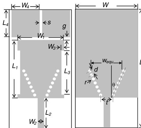
**Figure 1.** Geometry of the proposed directive SIW antenna.
