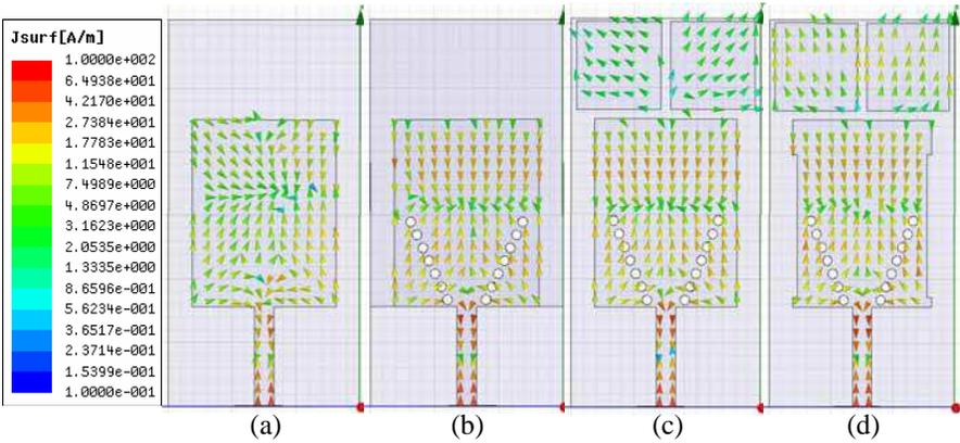
**Figure 3.** Simulated results of the surface current distributions at 4.8 GHz for the antenna studied in Figure 1, (a) initial patch only; (b) patch with via arrays; (c) patch with via arrays and parasitic elements; (d) patch with via arrays, parasitic elements, and sided slots.
