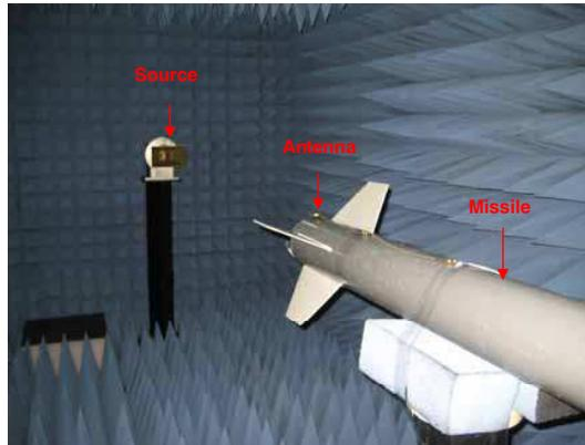
**Figure 8.** Photograph of experiment setup for the SIW antenna mounted on the scaled missile.
