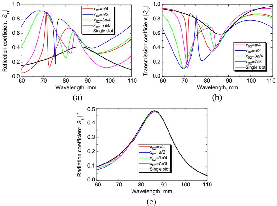
**Figure 2.** Energy characteristics of vibrators-slot system versus wavelength at  $x_{01} = a/8$ ,  $\tilde{Z}_{S1} = 0$ ,  $\tilde{Z}_{S2} = ikr_2 \ln(4.0)$ .
