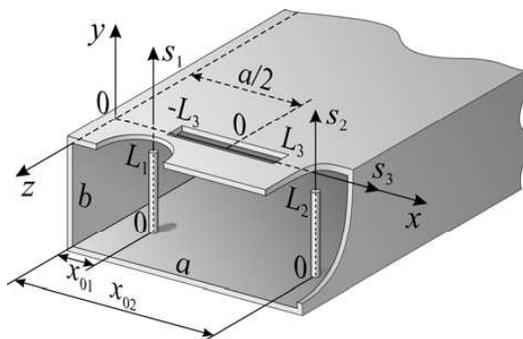
Figure 1. The geometry of the vibrator-slot structure and notations.
