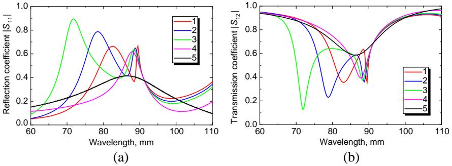
**Figure 3.** Energy characteristics of vibrators-slot system versus wavelength at  $x_{01} = a/8$ ,  $x_{02} = 7a/8$ ,  $\bar{Z}_{S1}(s_1) = ikr_1 \ln(4.0)\phi_1(s_1)$ : 1 —  $\bar{Z}_{S2} = ikr_2 \ln(4.0)$ ; 2 —  $\bar{Z}_{S2}(s_2) = ikr_2 \ln(4.0)\phi_2(s_2)$ ; 3 —  $\bar{Z}_{S2} = 0$ ; 4 — slot and one vibrator; 5 — single slot.
