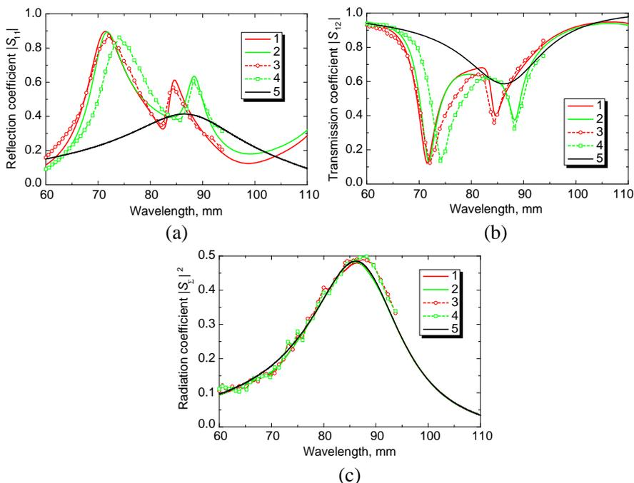
**Figure 5.** Energy characteristics of vibrators-slot system versus wavelength at  $x_{01} = a/8$ ,  $\bar{Z}_{S1} = 0$ ,  $x_{02} = 7a/8$ : 1 —  $\bar{Z}_{S2} = ikr_2 \ln(4.0)$ ; 2 —  $\bar{Z}_{S2}(s_2) = ikr_2 \ln(4.0)\phi_1(s_2)$ ; 3, 4 — experimental data (corrugated metallic conductors [12, 13]); 5 — single slot.
