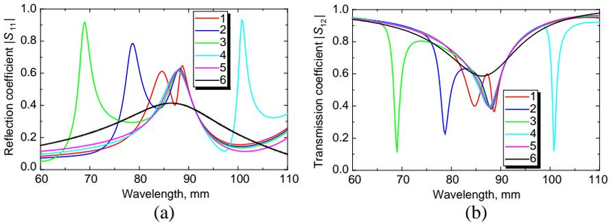
**Figure 4.** Energy characteristics of vibrators-slot system versus wavelength at  $x_{01} = a/8$ ,  $x_{02} = 15a/16$  (asymmetrical positions of vibrators),  $\bar{Z}_{S1}(s_1) = ikr_1 \ln(4.0)\phi_1(s_1)$ : 1 —  $\bar{Z}_{S2} = ikr_2 \ln(4.0)$ ; 2 —  $\bar{Z}_{S2}(s_2) = ikr_2 \ln(4.0)\phi_2(s_2)$ ; 3 —  $\bar{Z}_{S2} = 0$ ; 4 —  $\bar{Z}_{S2}(s_2) = ikr_2 \ln(8.0)\phi_1(s_2)$ ; 5 — slot and one vibrator; 6 — single slot.
