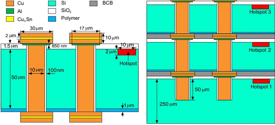
**Figure 1.** Cross-sectional view of single- and three-layer TTSVs in 3D integrated DRAM.
