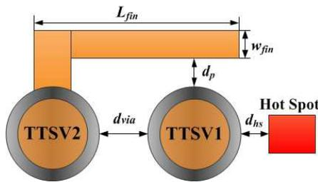
**Figure 2.** Top view of Fin structure ( $d_{via} = 5 \mu\text{m}$ ,  $d_p = 5 \mu\text{m}$ ,  $w_{fin} = 5 \mu\text{m}$ ,  $t_{fin}$  is the depth of Fin).
