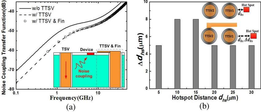
**Figure 3.** (a) Noise coupling transfer function of single-layer structure. (b) Compared to the case of TTSV without Fin, the distance that hot spot can be pulled away from the heat source when Fin structure is added to TTSV.
