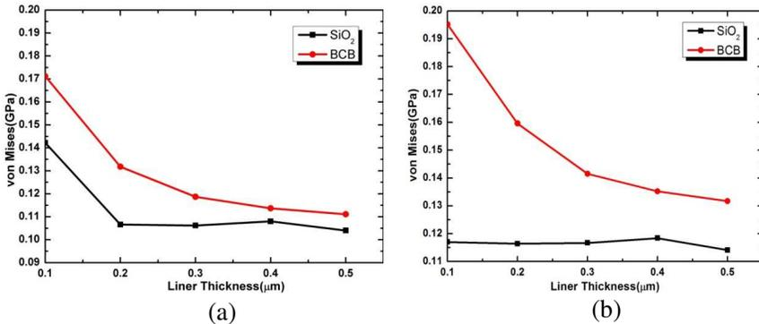
**Figure 11.** Maximum von Mises force of single-layer TTSV with  $\text{SiO}_2$  and BCB liner utilizing (a) temperature-independent and (b) temperature-dependent physical parameters.
