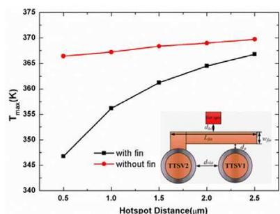
**Figure 4.** The maximum temperature of single-layer TTSVs varied with hotspot distance.
