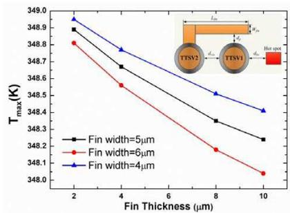
**Figure 5.** Maximum temperature of single-layer TTSV, with variation of Fin width and thickness.
