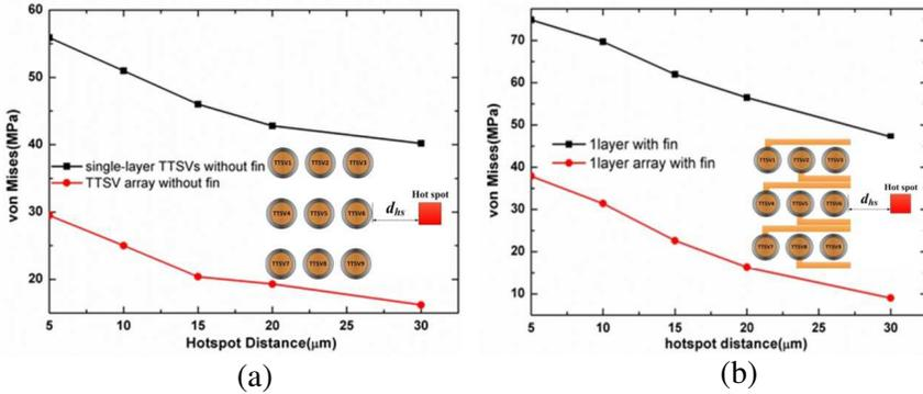
**Figure 10.** The maximum von Mises force of single TTSV and TTSV array (a) without and (b) with Fin.
