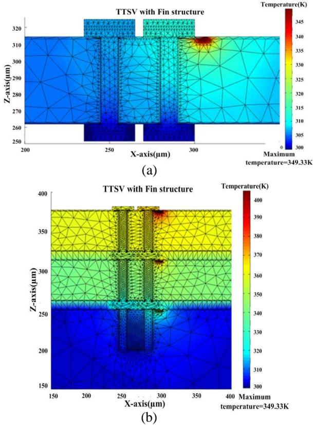
**Figure 7.** 3-D temperature distribution of (a) single- and (b) three-layer TTSVs. For single-layer TTSV,  $w_{fin} = 6 \mu\text{m}$  and  $t_{fin} = 10 \mu\text{m}$ ,  $d_{hs} = 10 \mu\text{m}$ , while  $t_{fin} = 2.65 \mu\text{m}$  and  $d_{hs} = 5 \mu\text{m}$  for three-layer case.
