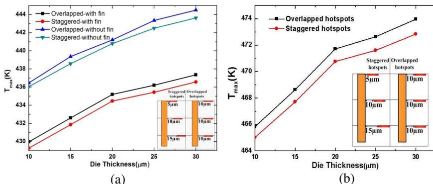
**Figure 8.** (a) Maximum temperature of three-layer TTSVs with overlapped and staggered hotspots. The case with and without Fin are considered. (b) Added with Fin structure, maximum temperature of three-layer TTSV with overlapped and staggered hotspots. The material properties are temperature dependent.
