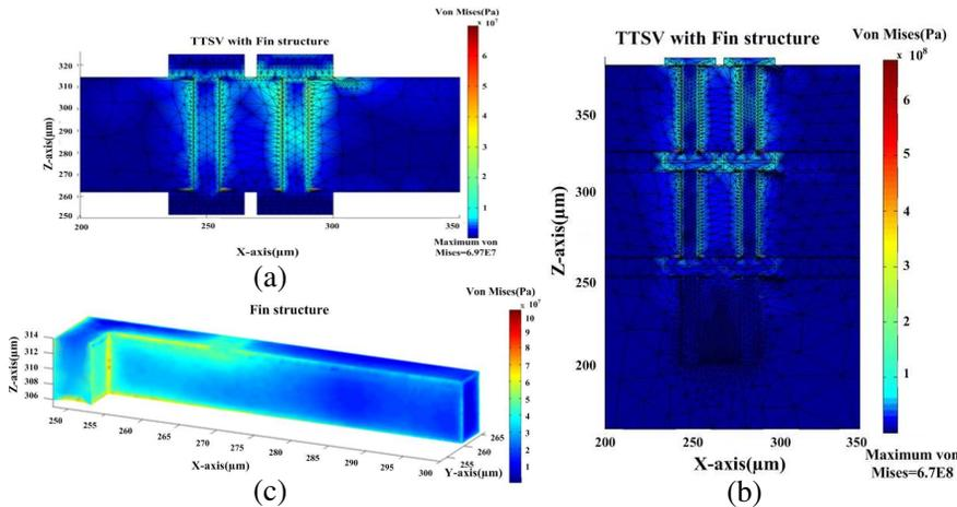
**Figure 9.** 3-D thermal stress distribution of (a) single- and (b) three-layer TTSVs. The geometry information and applied condition is the same as that in Fig. 7. The detailed thermal stress distribution of (c) Fin for single-layer TTSVs is provided, too.
