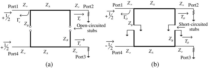
**Figure 2.** Equivalent model of the branch line coupler: (a) even mode, (b) odd mode.
