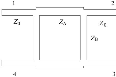
**Figure 1.** Geometry of the conventional coupler structure.
