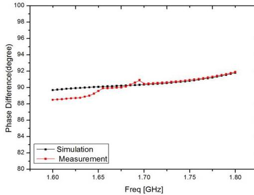
**Figure 8.** Phase difference between Ports 2 and 3.
