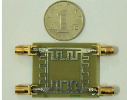
**Figure 6.** Fabricated proposed miniaturized coupler.
