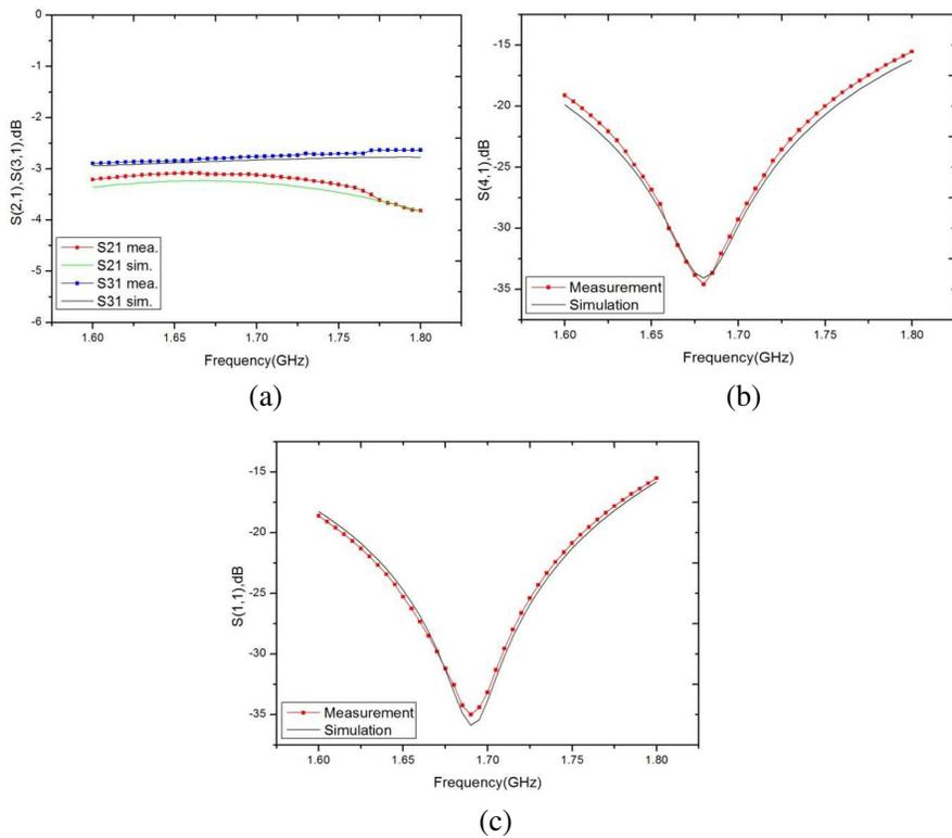
**Figure 7.** Simulation results: (a) magnitude of  $S(2,1)$  and  $S(3,1)$ , (b) magnitude of  $S(4,1)$ , (c) magnitude of  $S(1,1)$ .
