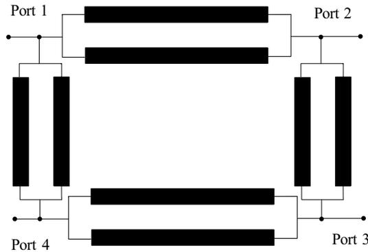
**Figure 4.** Equivalent circuit of the proposed coupler with dual transmission lines.
