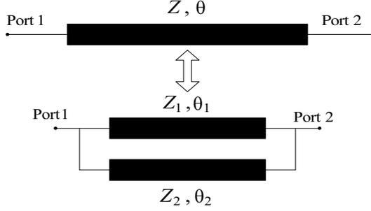
**Figure 3.** Equivalent circuit of single transmission line with dual transmission lines.
