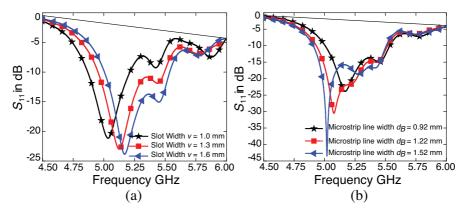
Figure 4. Slot and circular feeding line parameters effect on impedance band. (a)  $S_{11}$  with different slot width, when  $d_B = 0.92 \text{ mm}$ . (b)  $S_{11}$  with different circlular feeding line width, when v = 1.6 mm.
