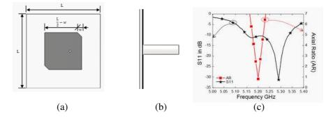
**Figure 1.** A basic truncated edge CP microstrip patch antenna. (a) Front view. (b) Side view. (c) Simulated  $S_{11}$  & AR for Ant.1.
