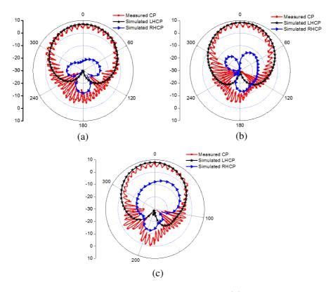
**Figure 10.** Radiation pattern at 5.20 GHz. (a) Ant.1 Simulated RHCP, LHCP & Measured at Phi =  $0^{\circ}$ . (b) Ant.2 Simulated RHCP, LHCP & measured at Phi =  $0^{\circ}$ . (c) Ant.3 Simulated RHCP, LHCP & Measured at Phi =  $0^{\circ}$ .
