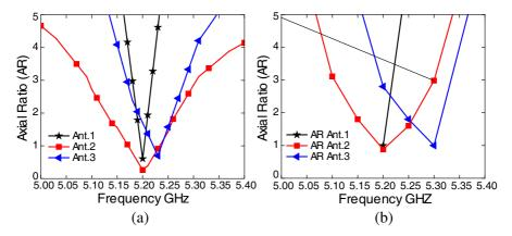
**Figure 9.** Axial ratio. (a) Simulated AR for fabricated antennas. (b) Measured axial ratio.
