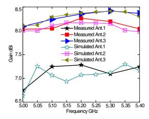
Figure 11. Simulated and measured gain to fabricated antennas.
