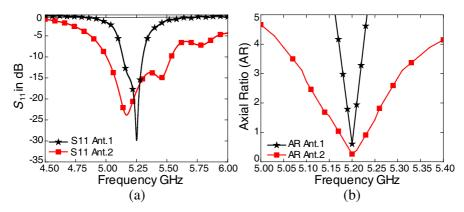
**Figure 5.** Simulated results of Ant.1 and Ant.2. (a)  $S_{11}$  Ant.1 VS Ant.2. (b) AR Ant.1 VS Ant.2.
