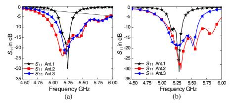
Figure 8. Simulated and measured return loss of fabricated antennas. (a) Simulated  $S_{11}$  for these 3 antennas. (b) Measured  $S_{11}$  compared among the three fabricated antennas.
