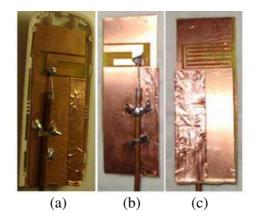
Figure 6. The fabricated antenna. (a) Monopole antenna without lower strip, (b) monopole antenna with lower strip and (c) bottom layer to show the meander strip.
