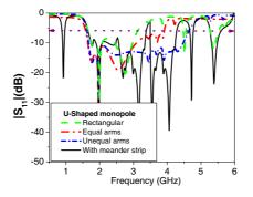
Figure 2. Simulated reflection coefficient of the design procedure.
