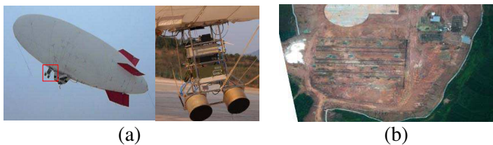
Figure 5. (a) Photos of the airship-mounted UWB SAR system; (b) Optical image of the area.
