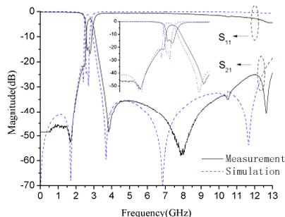
**Figure 6.** Comparison of simulated and measured frequency responses.
