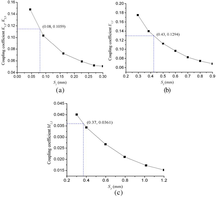
**Figure 3.** The extracting of coupling coefficients. (a)  $K_{1,2}, K_{2,3}$ . (b)  $E_{1,3}$ . (c)  $M_{1,3}$ .
