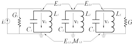
**Figure 1.** Equivalent circuit of three-order mixed-cross coupled filter.
