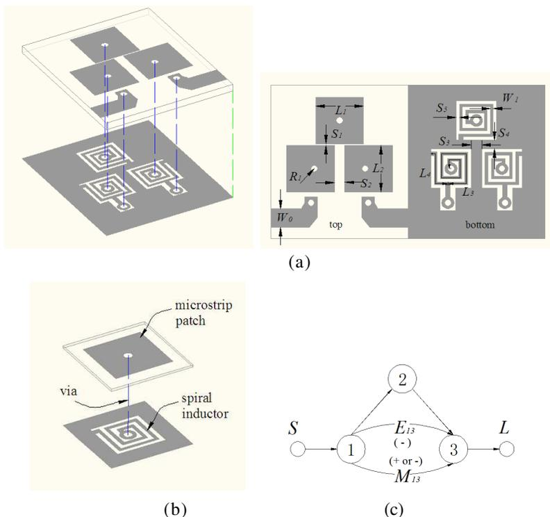
**Figure 2.** Three-order mixed-cross coupled filter. (a) Layout of proposed BPF. (b) Single PVS. (c) Corresponding coupling and routing scheme.
