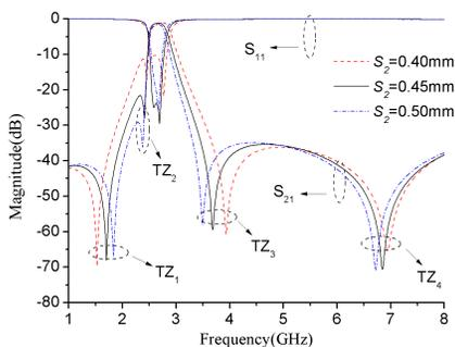
**Figure 4.** The simulation results and the impact of  $S_2$  to the filter responses.
