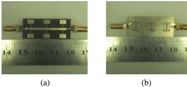
**Figure 6.** Structure of filter. (a) Top view. (b) Bottom view.
