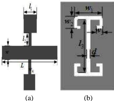
**Figure 2.** Structure of D-CRLH-TL. (a) Top view. (b) Bottom view.
