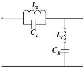
**Figure 1.** Equivalent circuit of D-CRLH-TL.
