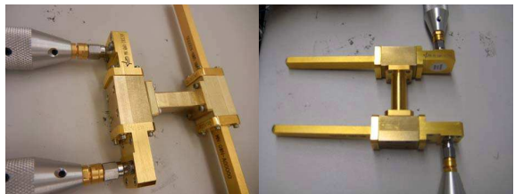
Figure 13. (a) Measurement for the return loss and isolation of one polarizer. (b) Measurement for the circular polarization.
