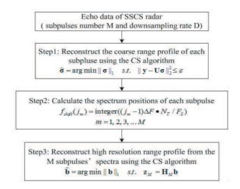
Figure 3. The flowchart of the CS-subaperture algorithm.
