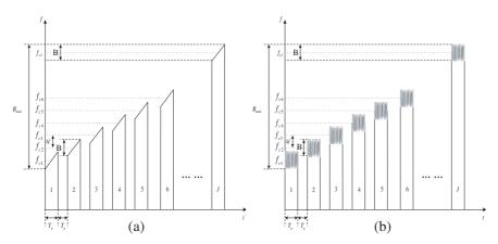
**Figure 1.** The conventional stepped frequency signal model. (a) Chirp signal as subpulse waveform; (b) chaotic signal as subpulse waveform. The subpulse number is J, the bandwidth of each subpulse is B, and the carrier frequency of *j*-th subpulse is  $f_{cj} = f_c + (j-1) \cdot \Delta f$ .
