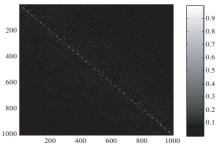
Figure 7. The column autocorrelation matrix. Each element is the scalar product of two columns in the sense matrix. Very good orthogonality is shown.
