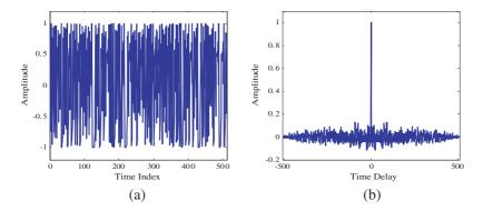
**Figure 5.** The improved Logistic-Map signal: (a) the real part; (b) the autocorrelation.
