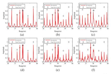
Figure 11. The result of subaperture algorithm with SSCS. (a), (b) and (c) are the results without filling the spectrum gaps, the corresponding subpulse number M are 16, 12, 8, respectively, while (d), (e), (f) are the results with spectrum gaps filled by super-SVA method, the corresponding subpulse number M are 16, 12, 8, respectively.
