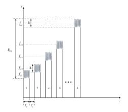
Figure 2. The sparse stepped chaotic signal (SSCS) model. It is constructed by randomly choosing M subpulses from the total J subpulses in Figure 1(b).
