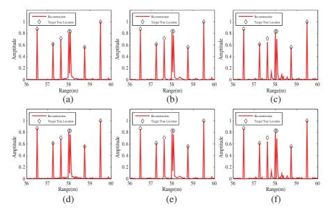
Figure 12. The results of CS-subaperture algorithm with SSCS with different subpulse number M and downsampling rate D. (a) M = 16, D = 5; (b) M = 12, D = 5; (c) M = 8, D = 5; (d) M = 16, D = 10; (e) M = 12, D = 10; (f) M = 8, D = 10.
