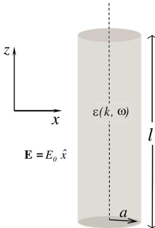
**Figure 1.** Schematics of a cylindrical nanowire of radius  $a$  with the axis oriented along the  $z$  axis characterized by a nonlocal dielectric function  $\varepsilon(k, \omega)$ . The external electric field oriented in  $x$  axis.
