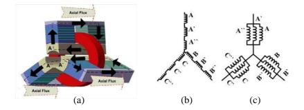
**Figure 1.** (a) The one-phase assembly of proposed machine without phase winding. (b) (c) Two possible winding configurations.
