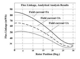
Figure 4. Flux linkage versus rotor position from analytical analysis.
