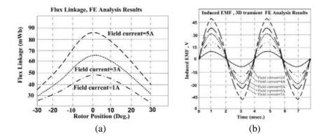
Figure 6. (a) Computed flux linkage for different rotor positions. (b) Computed induced Back-EMF from 3-D FE analysis for different rotor angles.
