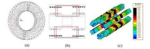
Figure 5. Magnetic flux density arrows for different parts of the proposed machine.
