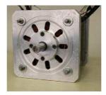
Figure 8. Proposed BLDC generator fabricated in the laboratory.
