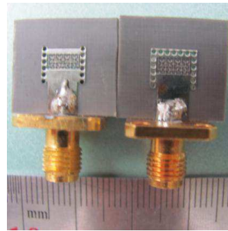
Figure 5. The fabricated prototypes of the fractal-based NOR antennas.
