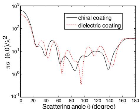
**Figure 4.** Comparison between the normalized differential scattering cross section  $\pi\sigma(\theta, 0)/\lambda^2$  for a chiral-coated conducting spheroid (solid line) ( $k_0a_1 = 6.28$ ,  $a_1/b_1 = 2$ ,  $k_0a_2 = 9.42$ ,  $a_2/b_2 = 2$ ,  $\varepsilon_r = 4$ ,  $\mu_r = 1$ ,  $\kappa = 0.5$ ) and that for the same model but with a dielectric coating (dotted line) ( $\kappa = 0$ ), both illuminated by an axial Gaussian beam of  $w_0 = 2\lambda$ .
