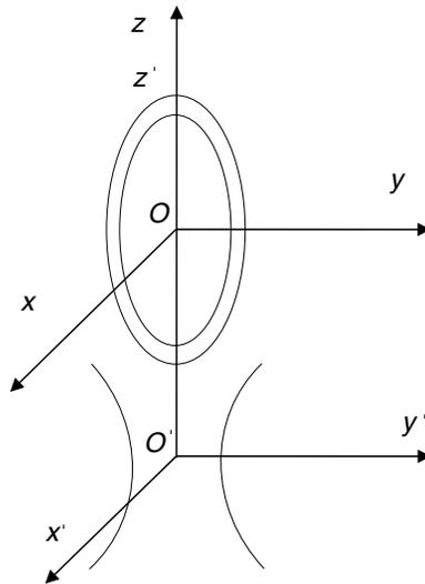
**Figure 1.** The Cartesian coordinate system  $Oxyz$  is obtained by a translation of the Gaussian beam coordinate system  $O'x'y'z'$  along the  $z'$  axis, and origin  $O$  is at  $(0, 0, z_0)$  in  $O'x'y'z'$ . A chiral-coated conducting spheroid is natural to  $Oxyz$ .
