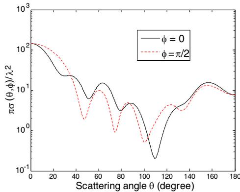
**Figure 2.** Normalized differential scattering cross sections  $\pi\sigma(\theta, 0)/\lambda^2$  and  $\pi\sigma(\theta, \frac{\pi}{2})/\lambda^2$  for a chiral-coated conducting spheroid ( $k_0a_1 = 6$ ,  $a_1/b_1 = 2$ ,  $k_0a_2 = 9.14$ ,  $a_2/b_2 = 2$ ,  $\varepsilon_r = 4$ ,  $\mu_r = 1$ ,  $\kappa = 0.5$ ) illuminated by an axial Gaussian beam with  $w_0 = 2\lambda$ .
