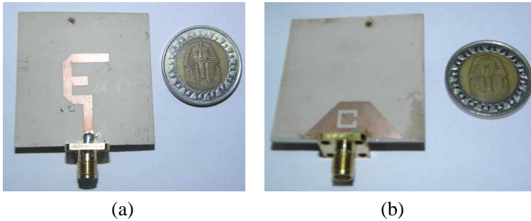
Figure 2. Photograph of fabricated E-shaped antenna. (a) Top view. (b) Bottom view.
