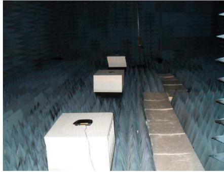
**Figure 1.** Experiment setup inside anechoic chamber.
