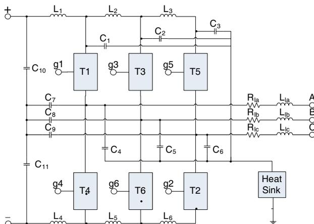
**Figure 6.** Three-phase inverter model with stray parameters.
