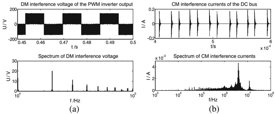
**Figure 11.** Simulation results. (a) Waveform and spectrum of DM disturbance voltage of the PWM inverter output. (b) Waveform and spectrum of CM disturbance currents of the DC bus.
