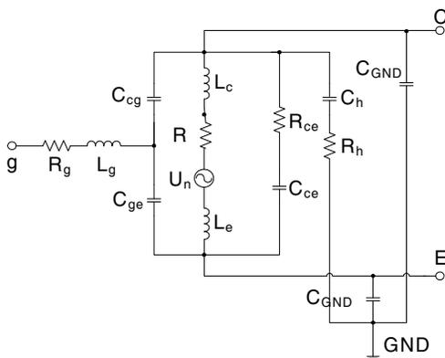
Figure 3. Stray parameters of IGBT.
