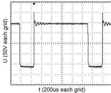
**Figure 2.** An experimental on-off waveform of IGBT.
