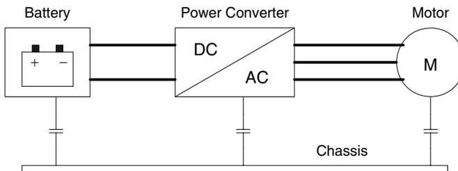
**Figure 1.** Electric drive system in electric vehicles.
