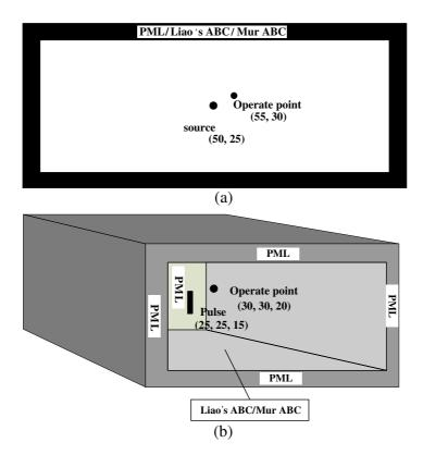
**Figure 1.** The model of the calculation domain. (a) The TE model in 2D grids (100 \* 50). (b) The model in 3D grids (50 \* 50 \* 30).
