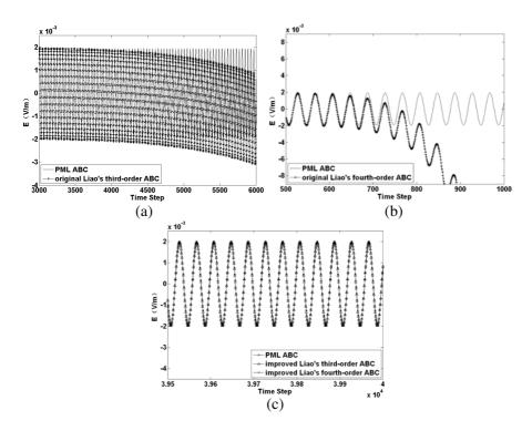
**Figure 3.** The electric field at the point (30, 30, 20) within the 50 \* 50 \* 30 cells 3D FDTD grid for different order Liao's ABC and 6-cell-thick PML ABC, plotted as a function of time step number. (a) Original Liao's third-order ABC and PML ABC in 3D. (b) Original Liao's fourth-order ABC and PML ABC in 3D. (c) Improved Liao's third-order, fourth-order ABC and PML ABC in 3D.
