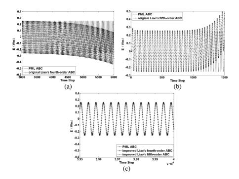
**Figure 2.** The electric field at the point (55, 30) within the 100 \* 50 cells 2D TE FDTD grid for different order Liao's ABC and 6-cell-thick PML ABC, plotted as a function of time step number. (a) Original Liao's fourth-order ABC and PML ABC in 2D. (b) Original Liao's fifth-order ABC and PML ABC in 2D. (c) Improved Liao's fourth-order, fifth-order ABC and PML ABC in 2D.
