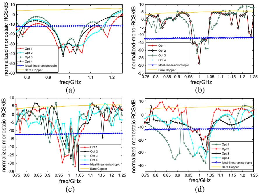
**Figure 2.** The monostatic echo widths of the optimized magnetic cloaks based on initial guesses of (a) simplified nonlinear cloak [18], (b) the ideal nonlinear cloak [1], (c) the nonlinear quasi-cloak [16], and (d) the default parameters provided by GA.
