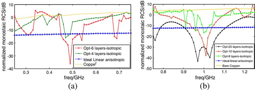
**Figure 5.** The monostatic echo widths from the optimized cloak realized by different number of layers. Target bandwidth 80 MHz at (a) 0.5 GHz, (b) 1 GHz. The echo widths from the ideal linear cloak, and the bare copper cylinder are presented as references.
