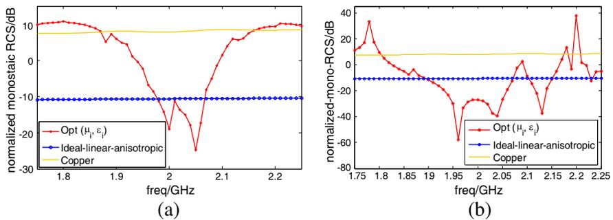
**Figure 6.** The monostatic echo widths from the optimized cloak designed using increased optimization parameters, with center frequency: 2 GHz, the ideal linear cloak, and the bare copper cylinder. (a)  $(\mu_i, \varepsilon_i)$ , (b)  $(\mu_i, R_i)$  are used as the optimization parameters.
