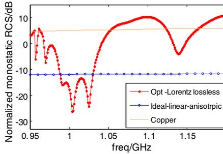
**Figure 7.** The monostatic echo widths from the optimized dispersive lossless cloaks, the ideal linear cloak, and the bare copper cylinder.
