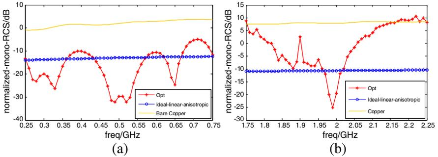
**Figure 4.** The monostatic echo widths from the optimized cloak targeting at 80MHz bandwidth with the same number of layers ( $M = 20$ ), the ideal linear cloak, and the bare copper cylinder. (a) Center frequency: 0.5 GHz. (b) Center frequency: 2 GHz.
