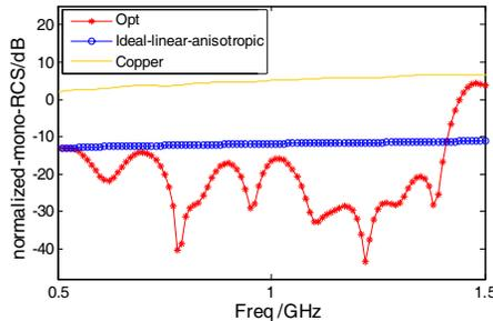
**Figure 3.** The monostatic echo widths from the optimized cloak targeting at 80% bandwidth, the ideal linear cloak, and the bare copper cylinder.
