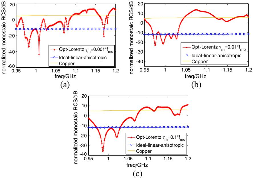
**Figure 8.** The monostatic echo widths from the optimized dispersive lossy cloaks, the ideal linear cloak, and the bare copper cylinder: (a)  $\gamma_m = 0.001 * f_{mo}$ ; (b)  $\gamma_m = 0.01 * f_{mo}$ ; (c)  $\gamma_m = 0.1 * f_{mo}$ .
