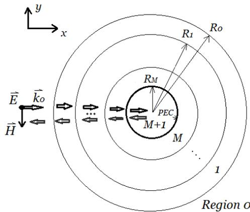
Figure 1. The cross section of an  $M$ -layered cylindrical structure.
