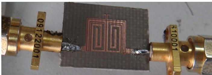
**Figure 4.** Photograph of the fabricated dual-passband filter.
