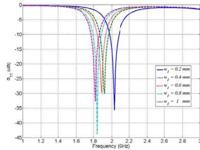
**Figure 5.** Reflection coefficient at port 1 of the modified patch crossover for different slot widths.
