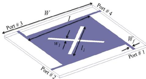
**Figure 3.** Modified crossover #1 using two perpendicular slots.
