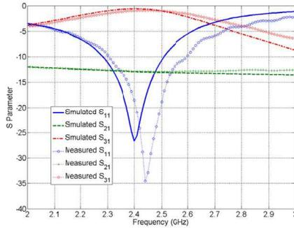
**Figure 11.** Simulated and measured  $S$  parameters of the reduced size square patch crossover.
