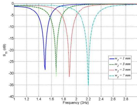
**Figure 7.** Reflection coefficient at port 1 of the modified patch crossover for different separation distances  $w_2$ .
