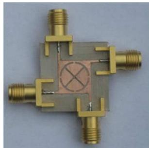
**Figure 10.** Fabricated prototype of the reduced size square patch crossover.
