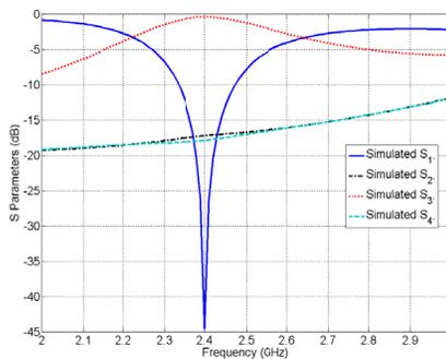
**Figure 2.** Simulated  $S$  parameters of the square patch crossover.
