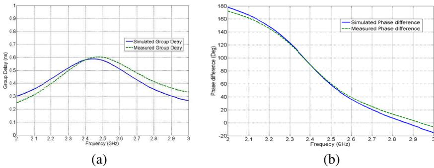
**Figure 12.** Reduced size square patch crossover (a) group delay and (b) transmission phase.
