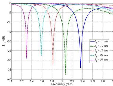
**Figure 4.** Reflection coefficient at port 1 of the modified patch crossover for different slot lengths.
