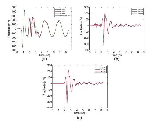
**Figure 3.** (a) All recorded signals. (b) All recorded signals after environment signal has been subtracted. (c) All signals after noise prior to first muscle wall reflection is removed.
