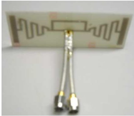
Figure 5. The two-port probe used to measure the input impedance of the tags under test.
