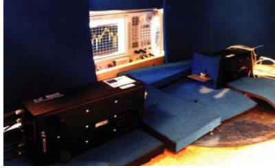
Figure 11. Cylindrical antenna measurement setup.
