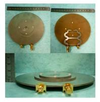
Figure 14. Top view, back view and side view of the proposed antenna.
