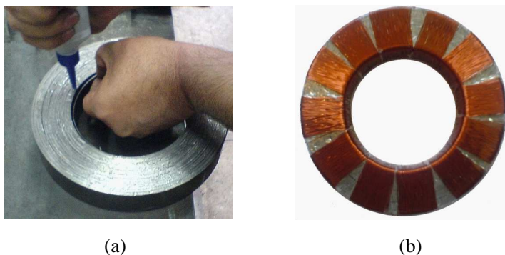
Figure 4. The stator of the prototype line-start axial-flux permanent-magnet motor. (a) Spiral laminated stator. (b) Stator winding is made of 12 coils with 90 turns each.
