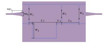
**Figure 4.** Layout of an in-line 3-pole generalized Chebyshev filter with one transmission zero using SIW technology. Cavity and coupling dimensions are measured from centre to centre of vias.
