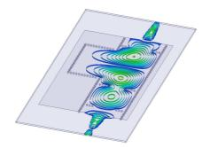
**Figure 5.** Electric field distribution of an in-line 3-pole generalized Chebyshev filter with one transmission zero using SIW technology at centre frequency.
