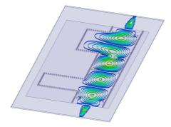
Figure 10. Electric field distribution in an in-line 5-pole generalized Chebyshev filter with two transmission zeros using SIW technology at centre frequency.
