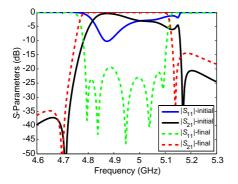
Figure 7. Scattering parameters for the initial dimensions  $(x_{str}$ in Table 2) and final dimensions  $(x_{opt}$  in Table 2) of a 5-pole generalized Chebyshev in-line SIW filter with two transmission zeros.
