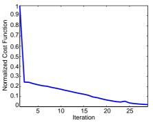
Figure 8. Convergence of the optimization routine for a 5-pole generalized Chebyshev filter with two transmission zeros.
