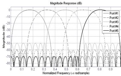
**Figure 3.** Magnitude response of  $1 \times 5$  band pass optical delay line filter.
