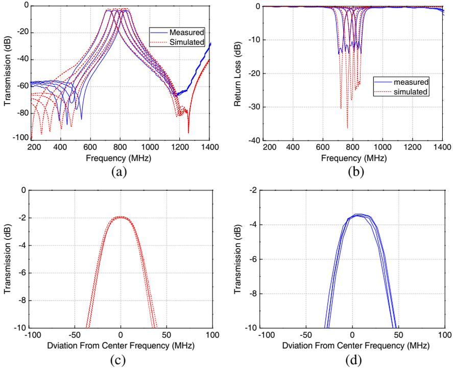
**Figure 3.** Simulated and measured results of the filter with 30-MHz bandwidth. (a)  $S_{21}$ . (b)  $S_{11}$ . (c) Superposition of the simulated passband responses. (d) Superposition of the measured passband responses.
