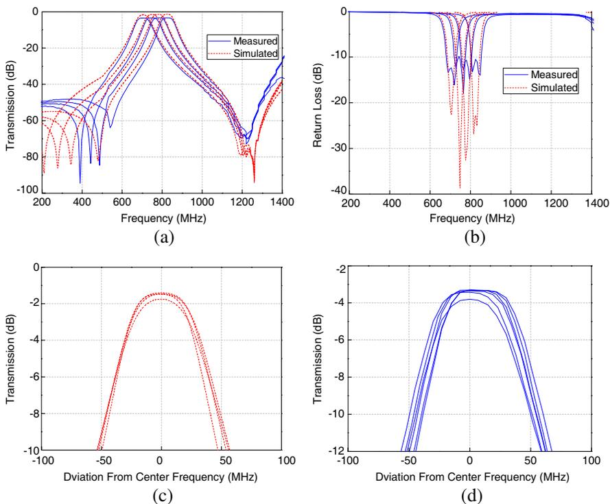
**Figure 4.** Simulated and measured results of the filter with 44-MHz bandwidth. (a)  $S_{21}$ . (b)  $S_{11}$ . (c) Superposition of the simulated passband responses. (d) Superposition of the measured passband responses.
