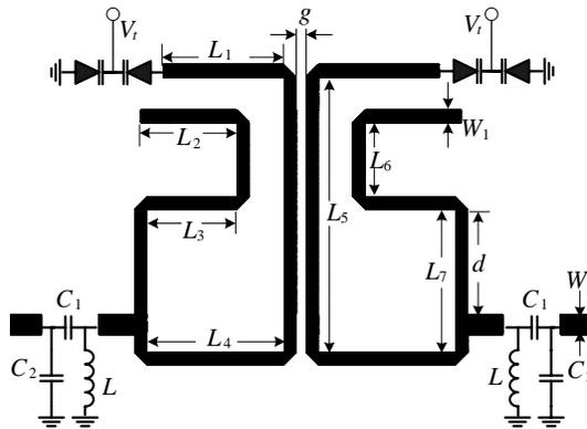
Figure 1. Layout of the proposed microstrip filter.
