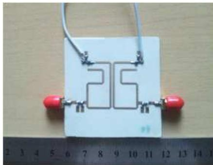
**Figure 2.** Photograph of the filter with 30-MHz bandwidth.
