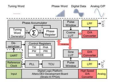
Figure 1. Proposed waveform synthesizer core.
