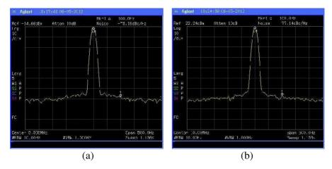
**Figure 5.** Calibration tone — phase noise. (a) Proposed RWS, (b) Agilent N8241A AWG.
