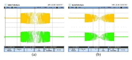
**Figure 7.** LFM waveform — time domain. (a) Proposed RWS, (b) Agilent N8241A AWG.
