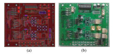
Figure 2. (a) HS-PCB layout design for HS-DAC board, (b) HS-DAC board
