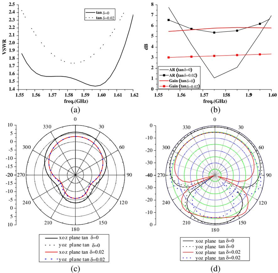
**Figure 3.** The simulated results of the designed antenna. (a) VSWR. (b) Gain and axial ratio. (c) Radiation pattern at 1.575 GHz. (d) Axial ratio pattern at 1.575 GHz.
