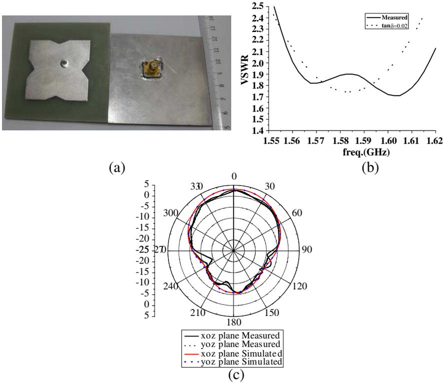
**Figure 10.** Photo of the fabricated antenna and the measured results. (a) Photo of the fabricated antenna. (b) Measured result of VSWR. (c) Measured results of circular polarization gain and radiation patterns.
