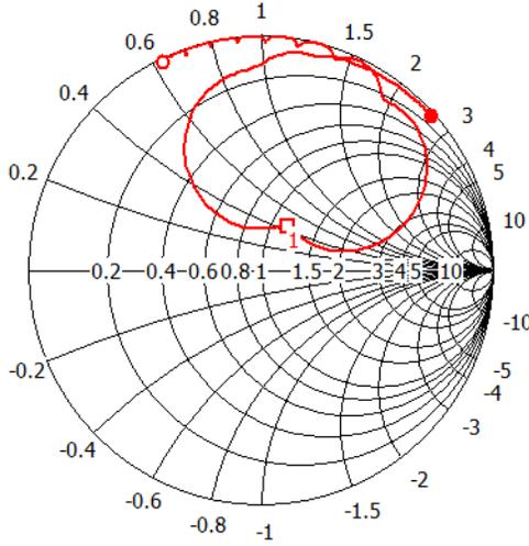
**Figure 2.** Simulated result of the input impedance (marker 1 is at a sharp point near the matching area. Two degenerate modes  $TM_{01}$  and  $TM_{10}$  are generated at this sharp point).
