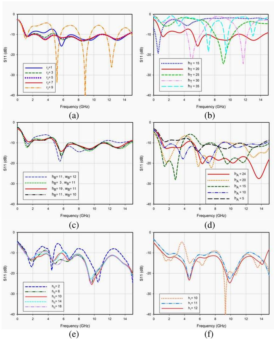
**Figure 3.** Simulated  $S_{11}$ -parameters of proposed antenna with various numbers of (a)  $r_2$ , (b)  $h_T$ , (c)  $h_B$ ,  $w_B$ , (d)  $h_A$ , (e)  $h_G$  and (f)  $h_1$  (the solid lines show the selected value for the desired parameters).
