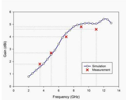
Figure 8. Simulated and measured gain of proposed antenna.
