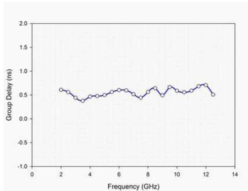
Figure 9. Measured group delay of proposed antenna.
