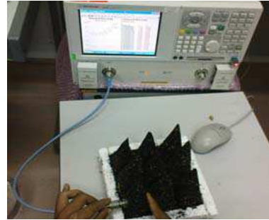
Figure 4. Defining the dielectric constant (real part, \epsilon'_r , and imaginary part, \epsilon''_r ) of the pyramidal microwave absorber using a dielectric probe.
