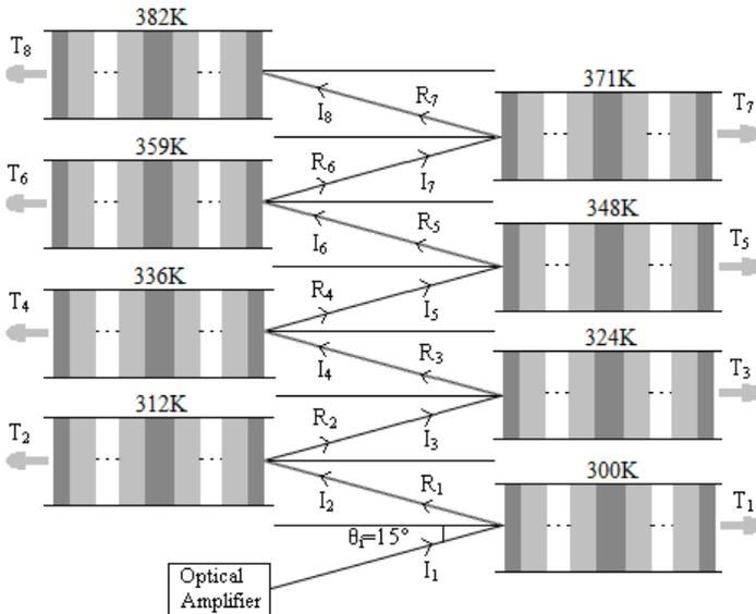
**Figure 1.** Proposed wavelength division demultiplexer based on one-dimensional photonic crystal with a defect.
