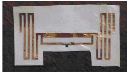
**Figure 6.** Conventional label-type tag used for comparison.
