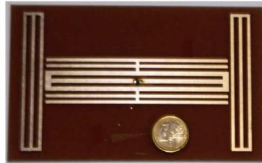
**Figure 2.** Prototype of the proposed tag.
