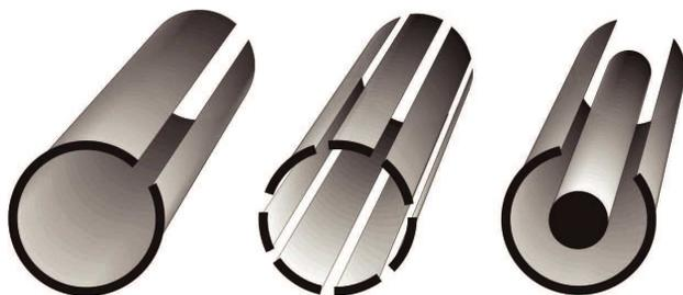
**Figure 1.** Geometry of a single slotted circular cylinder, multi-slotted circular cylinder and concentrically loaded slotted circular cylinder.
