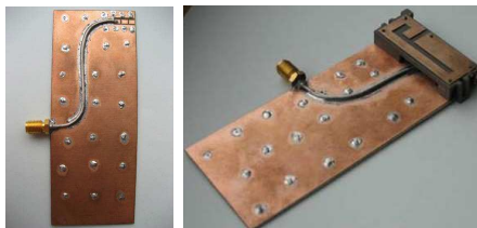
Figure 1. PIFA antenna for providing dual-band operation with dimensions W = 15 mm, L = 40 mm, and h = 6 mm over a ground plane of 100 mm \times 40 mm.
