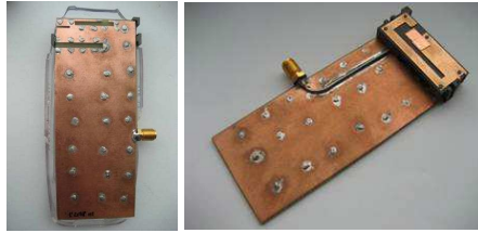
Figure 2. PIFA antenna with a slotted ground plane for providing hexa-band operation with dimensions W = 15 mm, L = 40 mm, and h = 6 mm over a slotted ground plane of 100 mm \times 40 mm.
