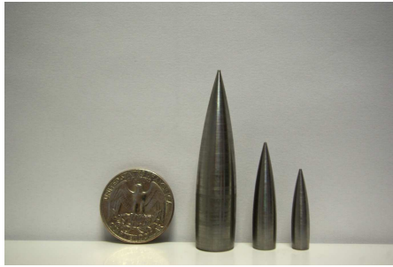
Figure 2. Photograph of the projectiles used for RCS measurement within an anechoic chamber, a quarter dollar coin is included for scale. The projectiles were made of steel and are representative of the shape and size of similar caliber military projectiles classed as small arms fire.
