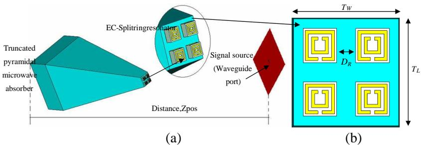
**Figure 5.** (a) The location of edge couple split ring resonator at the top of pyramidal microwave absorber (perspective view), Distance,  $Z_{pos} = 30$  cm, (b) The array of EC-SRR structure (plan view), distance between two SRR,  $D_r = 0.18$  cm, top length,  $T_L = 1$  cm, top width =  $T_W = 1$  cm.
