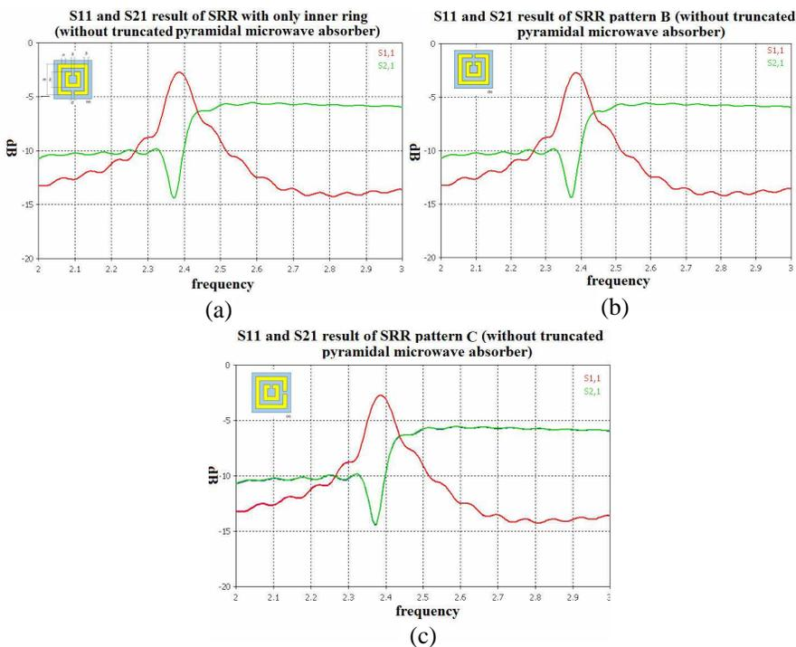
**Figure 6.** The  $S_{11}$  and  $S_{21}$  results for unit cell of EC-SRR designs (stand-alone SRR, without truncated pyramidal microwave absorbers): (a) SRR with only inner ring, (b) SRR Pattern A, (c) SRR Pattern B, (d) SRR Pattern C.
