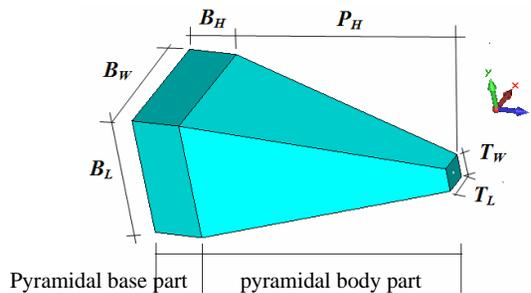
**Figure 4.** The dimensions of the truncated pyramidal microwave absorber; based length,  $B_L = 5$  cm, based width,  $B_W = 5$  cm, based height,  $B_H = 2$  cm, pyramid height,  $P_H = 13$  cm, top width,  $T_W = 1$  cm, and top length,  $T_L = 1$  cm.
