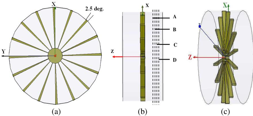
**Figure 1.** Simplified jet engine model. (a) Front view. (b) Side view. (c) 3-D engine view.
