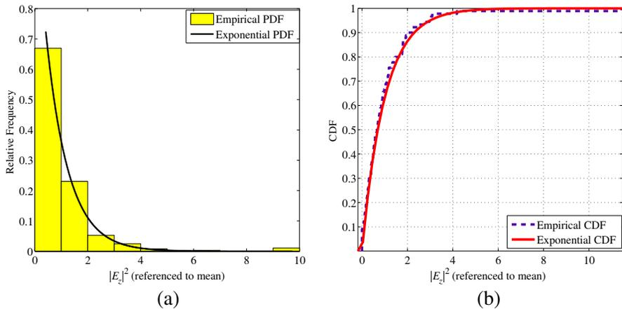
**Figure 2.** Data relative frequency histograms for the field along the cylindrical jet engine. (a) Empirical pdf versus theoretical pdf model. (b) Empirical cdf versus theoretical cdf models.
