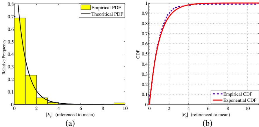
**Figure 3.** Data relative frequency histograms for the field at plane C. (a) Empirical pdf versus theoretical pdf model. (b) Empirical cdf versus theoretical cdf models.
